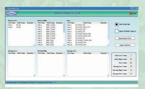
Interconnect test is like a board integrity check which checks for the interconnects that exist between various boundary scan device pins.
