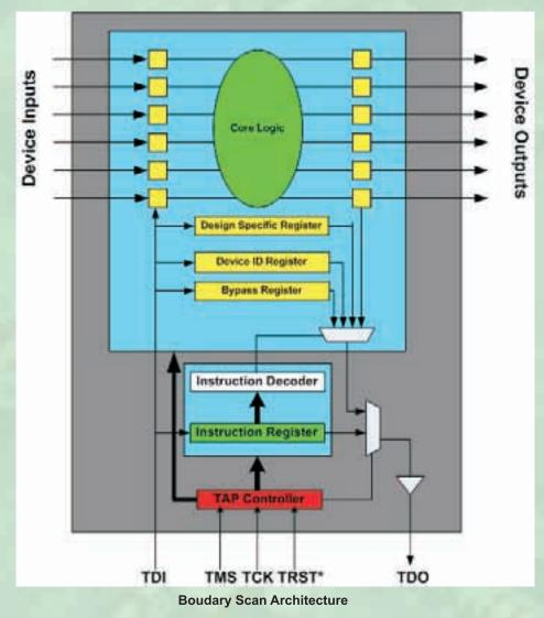
The IEEE1149.1 Standard Boundary Scan Chip Architecture facilitates application to perform
