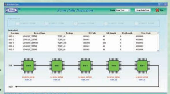
Scan Test performs a scan chain operation on a PCB to identify all the Boundary scan compatible devices available on board and the sequence in which they are connected to each other.
