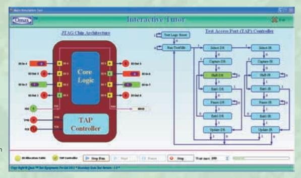
Interactive Tutor teaches users', the underlaying concept of Boundary scan and provides various simulations to strengthen their understanding.
