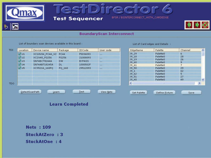
Boundary Scan Interconnect with Card Edge
