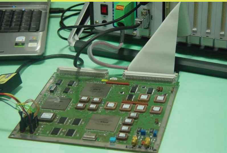
Boundary Scan Test done on a Radar Controller PCB
