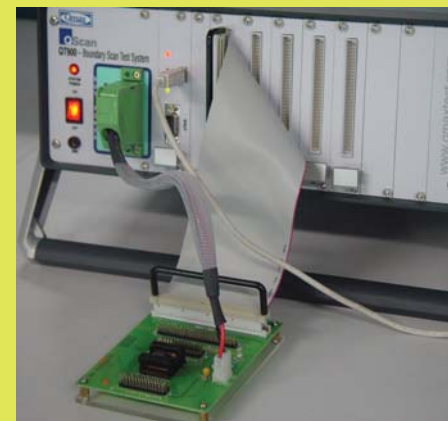
Testing of ICs in Out-Circuit mode using Qmax's QScan - Boundary Scan Test System
