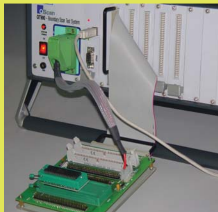
Testing of ICs in Out-Circuit mode using Qmax's QScan - Boundary Scan Test System
