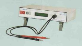
Offset switch to invoke the Offset mode, indicated by the offset symbol <>> in the display panel. Also used to control the volume of the audio tone indication in conjunction with Range Selector switch.
